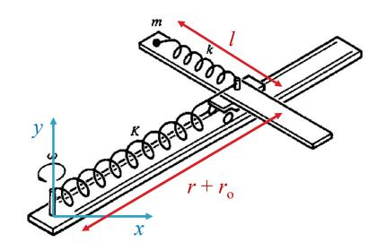
Point Transform between Lab and Rotating frames
